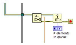
The consumer loop will only execute when data is present in the queue, so it does not require a Wait function. When the producer loop releases the queue, an error will appear in the consumer loop that stops it.
