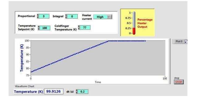
This VI must handle two new issues introduced by the magnitude and phase of the control signal: i) What to do when the amount of current demanded exceeds the capacity of the heater? ii) How to interpret a negative sign on the control signal, i.e. what causes the system to cool?
