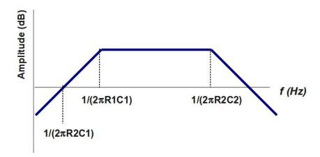
where the slopes are  $\pm 20$  dB/decade and the frequency axis is on a log10 scale. Determine values of R1, R2, C1, and C2 to set these frequency points at approximately 1 kHz, 10 kHz, and 100 kHz. The amplitude of the curve is not important; the goal is to obtain the desired frequency response. Calculate and display the amplitude and phase Bode plots of your design.
