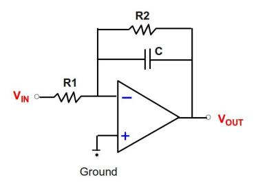
Launch the Bode analyzer and scan the frequency from 100 Hz to 20 kHz. This range corresponds to audio frequencies where the op-amp should behave ideally. If the ratio R2/R1 is increased significantly, however, this won't be the case. Confirm that you have low-pass filter behavior and save the data for later analysis.
