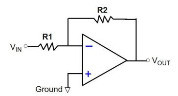
A circuit designer must be very careful with this formula. It suggests that any amount of gain can be attained by adjusting the resistor ratio. In addition, the simple formula ignores complications introduced by operating at high frequencies.
