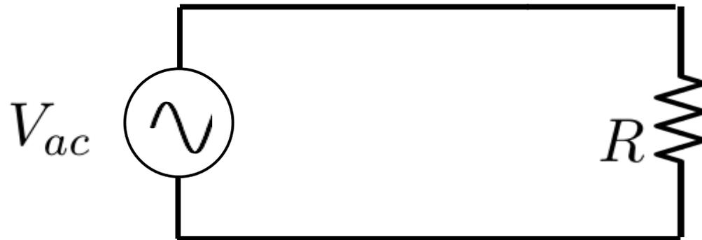
$$\text{POWER} = \frac{V_{ac}^2}{R} = \frac{V_p^2}{2R} \Rightarrow V_{RMS} = \frac{V_p}{\sqrt{2}}$$
