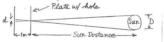
Then adjust the distance between the two plates to be some known distance,  $e.g.\ 1$  m, and measure the diameter, d, of the Sun's image on the "other" plate. If you measure, d, in inches, or millimeters, etc you need to convert it to meters! Curiously you have measured the angular diameter of the Sun:
