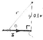
9&10] What is the magnetic field caused by a 0.1 m straight segment of wire carrying a 60 A current, at a point 0.1 m away from the end as shown?
