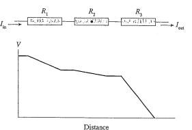
b. Rank in order, from largest to smallest, the three resistances  $R_1$ ,  $R_2$ , and  $R_3$ .
