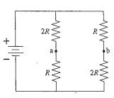
b. If a wire is connected between points a and b, does a current flow through it? If so, in which direction—to the right or to the left? Explain.
