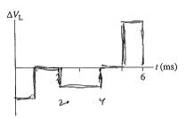
23. The figure shows the potential difference across an inductor. There is no current at t = 0. Draw a graph of the current through the inductor as a function of time. There are no numbers, but your graph should have the correct shape and proportions.
