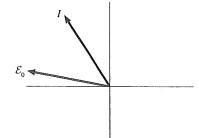
20. The resonance frequency of a series *RLC* circuit is greater than the emf frequency. Does the current lead or lag the emf? Explain.
