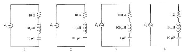
Rank in order, from largest to smallest, the maximum currents  $(I_{\text{max}})_1$  to  $(I_{\text{max}})_4$ .
