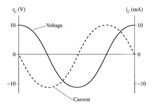
7. A 13  $\mu$ F capacitor is connected to a 5.5)/250 Hz oscillator. What is the instantaneous capacitor current  $i_C$  when  $\mathcal{E} = (-5.5)$
