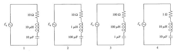
Rank in order, from largest to smallest, the maximum currents  $(I_{max})_1$  to  $(I_{max})_4$ .
