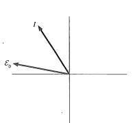
20. The resonance frequency of a series RLC circuit is greater than the emf frequency. Does the current lead or lag the emf? Explain.
