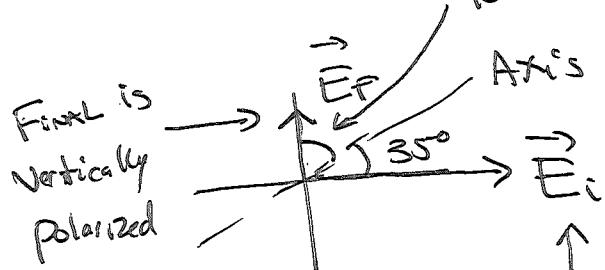
initially Beam is Horizontally polarized
