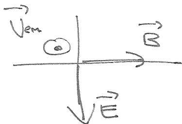
RHR  $\Rightarrow$  initially  $\vec{E}$  must point downwards so that when we curl from  $\vec{E}$  to  $\vec{B}$ , our thumb points out of page
