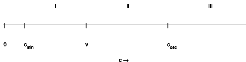
FIG. 3. Regions of the wave-front speed c . The speed cannot be lower than c_{min} . Solutions have different shapes according to whether c lies between c_{min} and the medium dictated speed v , between the latter and c_{osc} , larger than c_{osc} , or on the boundaries separating these regions. The explicit expressions are displayed in the text in reference to these regions.
